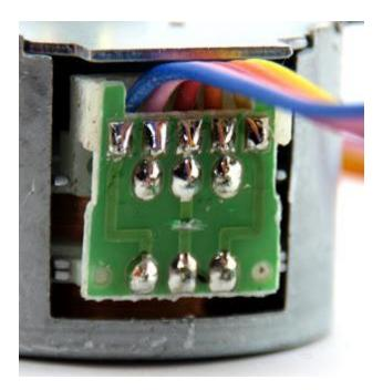
This is what the PCB looks like in detail. The red connection in the scheme above is actually the copper connection in this picture that I cut with a cutter knife. That's all you need to do! Well, for your own peace of mind, you could also try to re-attach the blue plastic cover. And now, ignore the red wire of the motor. We don't need it anymore.
